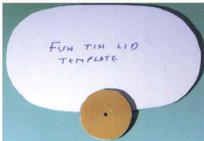
Fig. 2: Illustrating the template (recommended) to be used for cutting the shape of the main p.c.b., along with a tuning dial 'scribed' from SRPB material (see text).
