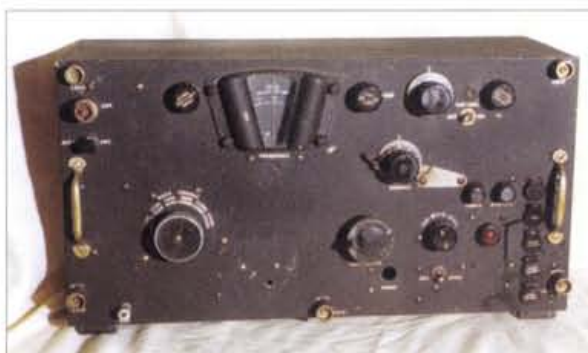
Fig. 2: The BC-312 receiver, main tuning lower centre right with the receiver fine tuning above it. There is a name plate missing from just below the dial (See text).
