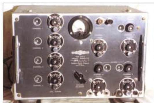
Fig. 1: The TA-12 transmitter, the four oscillators are situated down the left side, with the p.a. controls on the right and band changing controls in the centre (see text).
