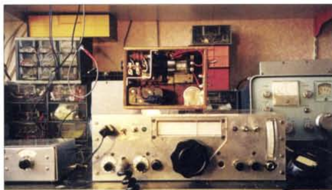
Fig. 4: Inside the 'One Valve Midget Portable' receiver from the October 1945 issue of PW . It gives a good account of itself, in spite of having only one active device.
